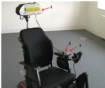
Figure 8. The prototype 1-headrest sensor plate; 2-reverse button; 3-LCD for reference information
